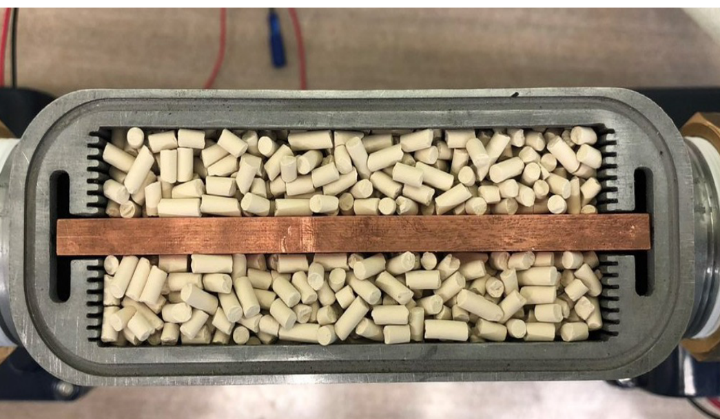
Inside view of the RCAP, showing zeolite pellets, copper heat exchange plate, and RCAP housing
